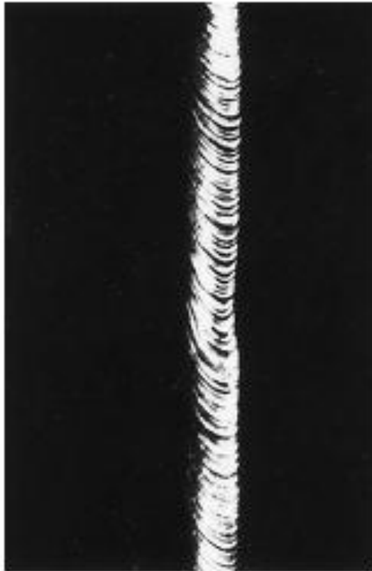
Figure 7.9 Slip in a zinc single crystal. (From C. F. Elam, The Distortion of Metal Crystals , Oxford University Press, London, 1935.)
