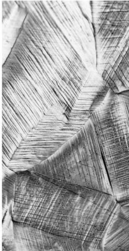
Figure 7.10 Slip lines on the surface of a polycrystalline specimen of copper that was polished and subsequently deformed. 173 \times . [Photomicrograph courtesy of C. Brady, National Bureau of Standards (now the National Institute of Standards and Technology, Gaithersburg, MD).]
