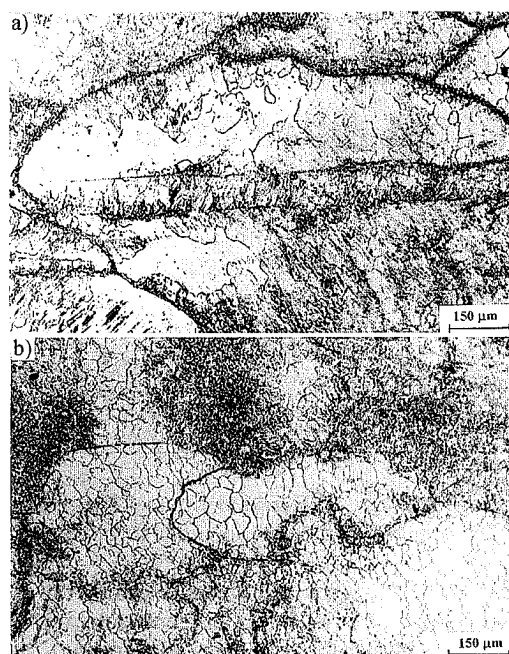
Fig. 8. AISI 304 (8a) and AISI 304L (8b) steels in the (S+P) condition, 60 % deformed and annealed at 750°C - 1 h. Optical Microscopy. Electrolytic etching in 30 % nitric acid and water. The "old" (prior) grain boundaries were decorated by the M_{23}C_6 precipitation.
